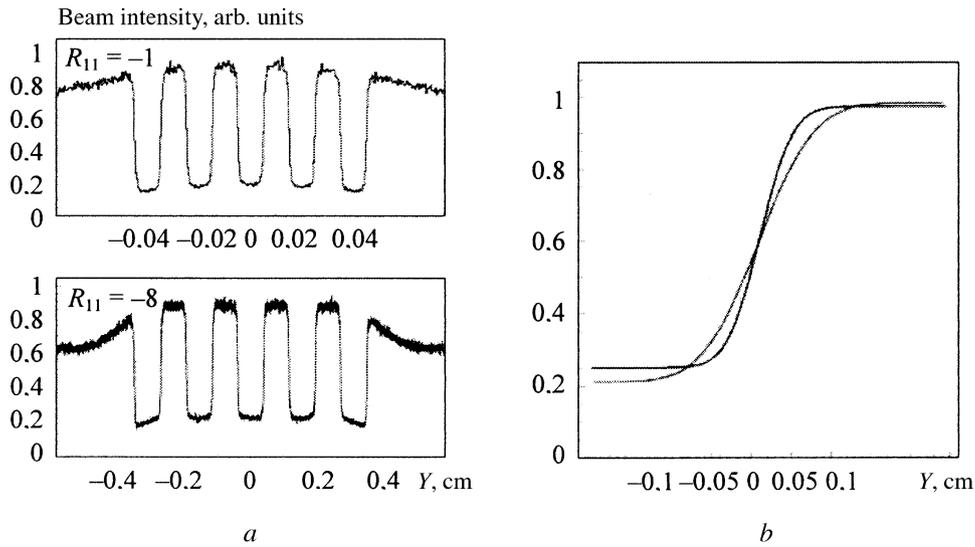
Fig. 6. Resolution of magnetic optics systems  $-8$  and  $-1$  of the setup for a periodic copper test object.
