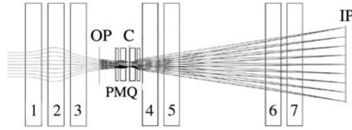
Fig. 3. Arrangement of the magnetic components and the proton trajectories in the channel of a proton radiographic facility with image transmission coefficient  $-8$ .
