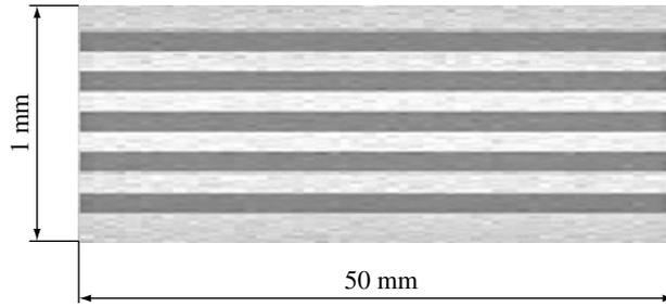
Fig. 5. Simulation of a proton radiographic image of a periodic 5 mm thick (in the beam direction) copper test structure. The image corresponds to five pairs of lines per 1 mm for the system  $-1$ .
