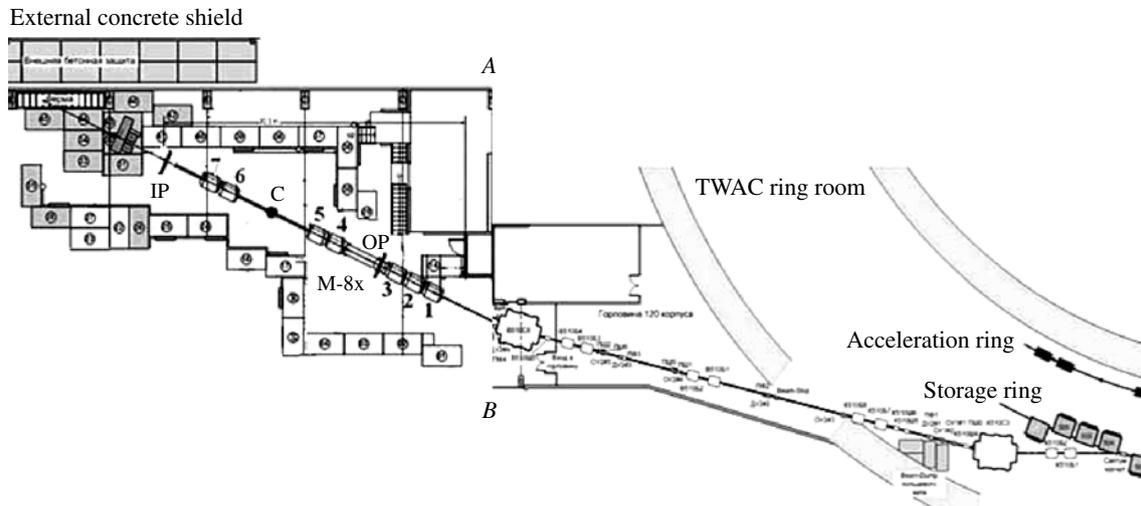
Fig. 1. Arrangement of the magnetic components, forming a proton beam for radiographic experiments, and quadrupole lenses of the proton radiography facility in the TWAC accelerator.
