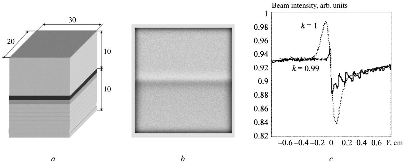
Fig. 7. Model of a detonation wave: *a*) simulation of a proton radiographic image for the system –1; *b*) image in the image plane; *c*) profile of the image along the vertical direction ( $k$  – correction factor for the magnetic field).
