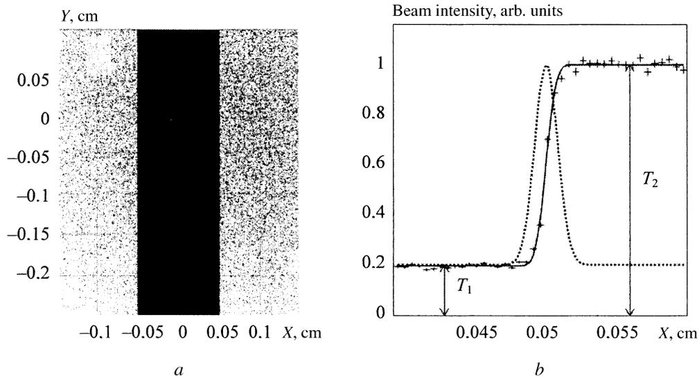
Fig. 4. Model of the test object “sharp boundary”: *a*) simulation of the proton radiographic image for the system  $-1$ ; *b*) horizontal profile of the right-hand boundary in the interval  $-0.5 < y < 0.5$  (+) and results of fitting a Gaussian distribution (•).
