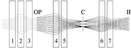
Fig. 2. Arrangement of the magnetic components and the course of the proton rays of the channel of the proton radiographic facility with image transmission coefficient  $-1$ .
